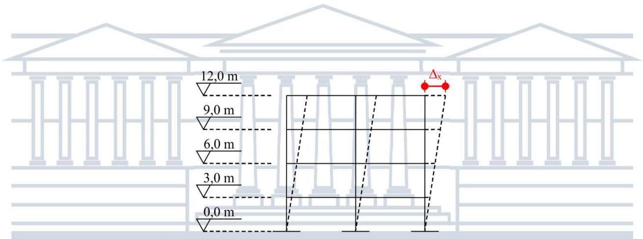
$$M_{1,tot,d} = \frac{(q)_{d,v\text{ento}} \times \ell^2}{2} = \frac{4,2 \times 12^2}{2} = 302,4 \text{ kNm} = 302\,400 \text{ kNmm}$$
